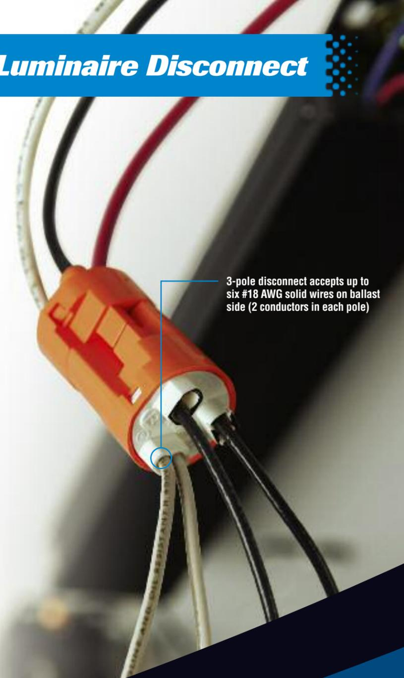
3-pole disconnect accepts up to six #18 AWG solid wires on ballast side (2 conductors in each pole)
