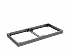
**Description:** Acts as a stabiliser when cabling is routed between bayed enclosures. With the PCP, plinths can be combined and fixed to the floor before the enclosures are mounted on them. The PCP can be used when cables have to go under the enclosure. For 200 mm high plinths, the PCP can be mounted in three different heights, top, middle or bottom. The hole pattern for cage nuts and M5x10 screws, allows accessories to be mounted.
