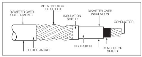
Figure 4. Illustration showing typical construction of high voltage underground cable.
