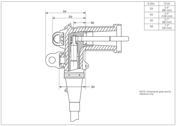
Figure 3. Elbow profile and stacking dimensions as referenced in IEEE Std 386<sup>TM</sup> standard.
