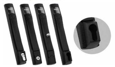
Flush Handles are optional for any solid, window or disconnect door that includes 3-point latching, except Voice/Data and Colocation cabinets. They are ergonomically designed to provide style and function in a low profile. The handle is die-cast zinc finished with RAL 9005 textured black polyester powder paint. Provision to add your logo is included. Handle can be installed to rotate either clockwise or counterclockwise.
