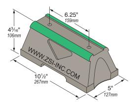
The CBN-Base Rooftop Support is UV resistant and suitable for installation on most types of roofing material or other flat surfaces. Can be used as a curb (sleeper) replacement. Screw fasteners can be used to attach one or two hole pipe straps or a piece of strut (not included).
