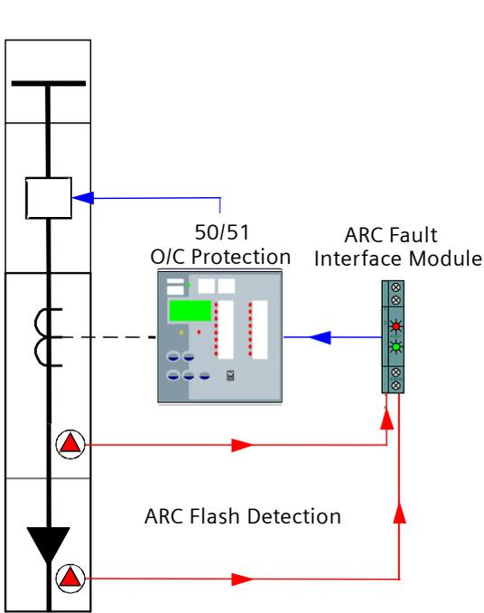
Figure 1: Cable box and CT chamber protection
