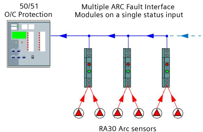
Figure 3: Multiple Arc Modules per status input
