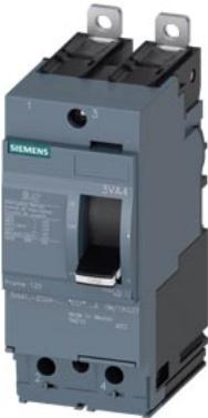
circuit breaker 3VA4 UL Frame 125 breaking capacity class M 35 kA @ 480 V 2-pole, line protection TM210, FTFM,  $I_n=20$  A overload protection  $I_r=20$  A permanently set short-circuit protection  $I_s=15 \times I_n$  in terminal connection
