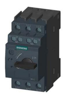
CIRCUIT-BREAKER SZ S00, FOR MOTOR PROTECTION, CLASS 10, A-REL.1.1...1.6A, N-RELEASE 21A, SCREW CONNECTION, STANDARD SW. CAPACITY, W. TRANSVERSE AUX. SWITCH 1NO+1NC
