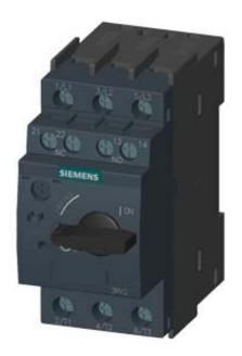
CIRCUIT-BREAKER SZ S00, FOR MOTOR PROTECTION, CLASS 10, A-REL. 0.14...0.2A,N-REL.2.6A, SCREW CONNECTION, STANDARD SW. CAPACITY, W. TRANSVERSE AUX. SWITCH 1NO+1NC
