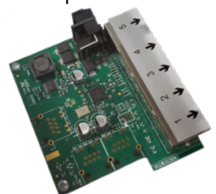
Ethernet Node Switch Expansion
