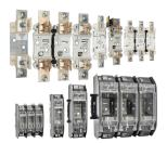
NH fuse-bases are available for delivery in single-pole and three-pole designs and can be closely mounted in parallel rows. Each three-pole base is upplied with two phase-partition walls. NH fuse-links plugon covers which clip onto the contact springs can also be supplied for these bases.
