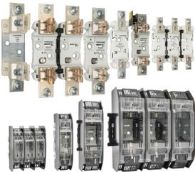
NH fuse-bases are available for delivery in single-pole and three-pole designs and can be closely mounted in parallel rows. Each three-pole base is supplied with two phase-partition walls. NH fuse-links plug on covers which clip onto the contact springs can also be supplied for these bases.
