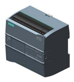
SIMATIC S7-1200, CPU 1214C, COMPACT CPU, AC/DC/RLY, ONBOARD I/O: 14 DI 24V DC; 10 DO RELAY 2A; 2 AI 0 - 10V DC,
