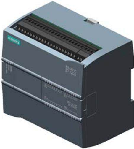
SIMATIC S7-1200, CPU 1214C, CPU COMPACTA, DC/DC/DC, E/S INTEGRADAS: 14 DI 24V DC; 10 DO 24 V DC; 2 AI 0 - 10V DC, ALIMENTACION: DC 20,4 -28,8 V DC, MEMORIA DE PROGRAMA/DATOS 75 KB
