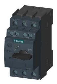
CIRCUIT-BREAKER SZ S0, FOR MOTOR PROTECTION, CLASS 10, A-RELEASE 14...20A, N-RELEASE 260A, SCREW CONNECTION, STANDARD SW. CAPACITY, W. TRANSVERSE AUX. SWITCH 1NO+1NC
