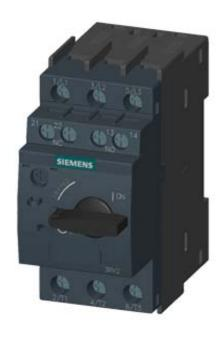
CIRCUIT-BREAKER SZ S00, FOR MOTOR PROTECTION, CLASS 10, A-RELEASE 7...10A, N-RELEASE 130A, SCREW CONNECTION, STANDARD SW. CAPACITY W. TRANSVERSE AUX. SWITCH 1NO+1NC
