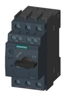
CIRCUIT-BREAKER SZ S00, FOR MOTOR PROTECTION, CLASS 10, A-RELEASE 4.5...6.3A, N-RELEASE 82A SCREW CONNECTION, STANDARD SW. CAPACITY W. TRANSVERSE AUX. SWITCH 1NO+1NC
