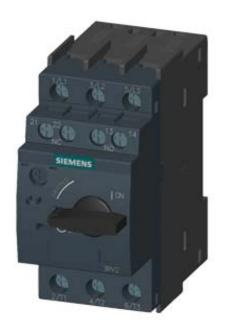
CIRCUIT-BREAKER SZ S00, FOR MOTOR PROTECTION, CLASS 10, A-RELEASE 2.8...4A, N-RELEASE 52A, SCREW CONNECTION, STANDARD SW. CAPACITY, W. TRANSVERSE AUX. SWITCH 1NO+1NC
