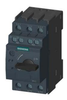
CIRCUIT-BREAKER SZ S00, FOR MOTOR PROTECTION, CLASS 10, A-REL. 1.8...2.5A, N-RELEASE 33A SCREW CONNECTION, STANDARD SW. CAPACITY, W. TRANSVERSE AUX. SWITCH 1NO+1NC
